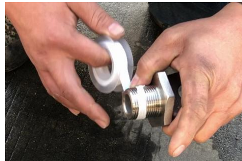
Step 2 Seal the Drag End Accessories with sealing tape.
