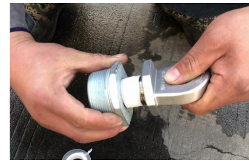
Step 3 Drag end accessories connect to Reducing Joint.
