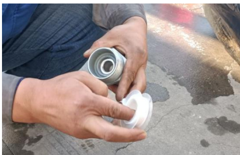
Step 1 Twine sealing tape on Reducing Joint.
