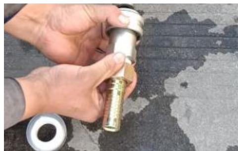
Step 6 Quick Connectors B connect with Hose Fitting. With sealing tape.
