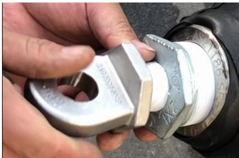
Step 5 Reducing Joint connect to airbag end.
